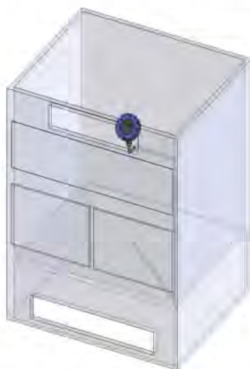
Figure 3. Guided wave in a stainless steel bin.
