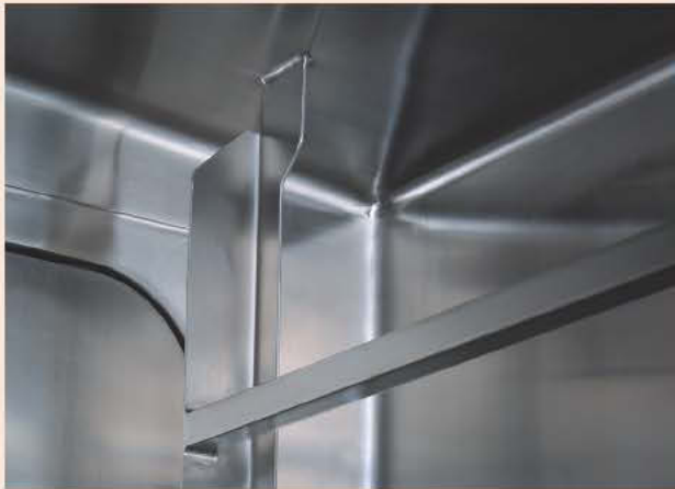
Figure 1 | Pharmaceutical-grade washer chamber with large radius, round corners
