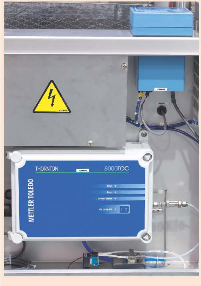
Figure 4 Online TOC monitoring system used in pharmaceutical-grade washers to measure the level of organic residues left in final rinse water
