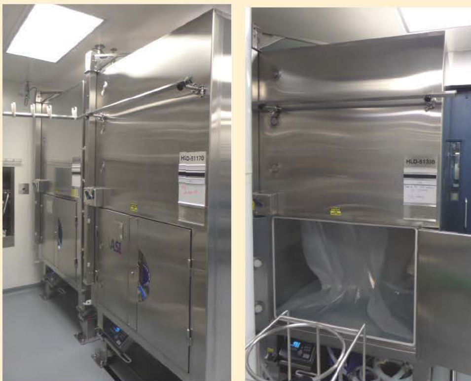
Figure 1 Large-scale disposable process solution storage tote and defined tubing routing
