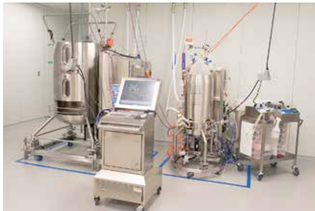
One of two pairs of 50- and 500-liter bioreactors with a common HMI
