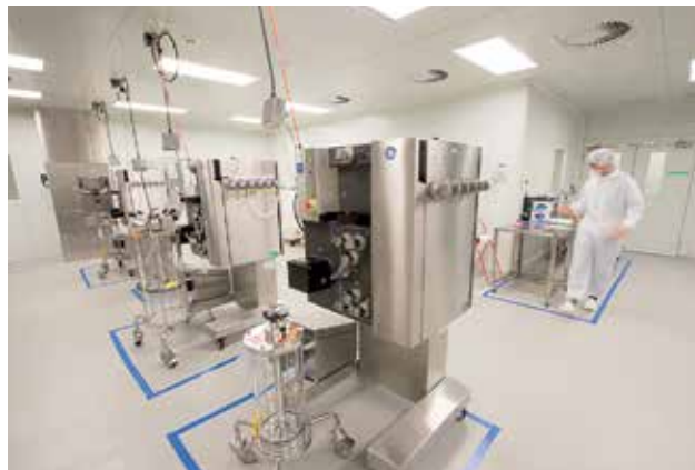
Purification room with three chromatography systems set up with reusable columns
