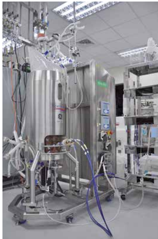
50-liter XDR bioreactor supplied in June 2013
