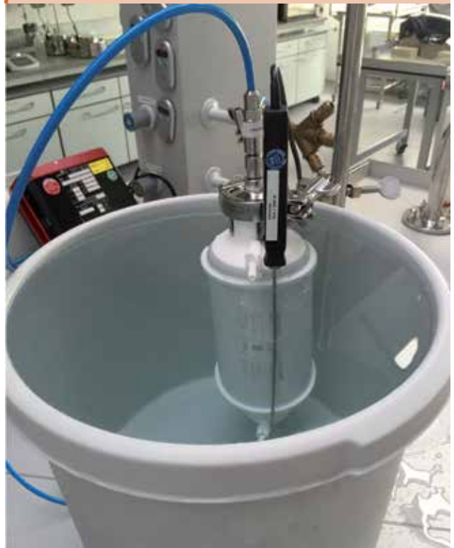
Figure 1: 10-inch filter capsule with attached temperature sensor
