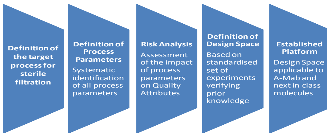
Figure 5.8 Schematic of the steps presented to establish a sterile filtration process platform and apply it to A-Mab.
